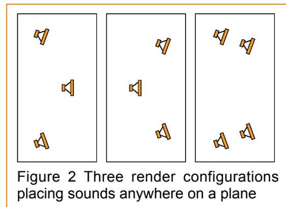
By feeding separate channel signals to the loudspeakers at the render area extremities it would thus be possible to place sounds at any distance in any direction on the plane between the two lines formed by the arrays, and feed the corresponding common
