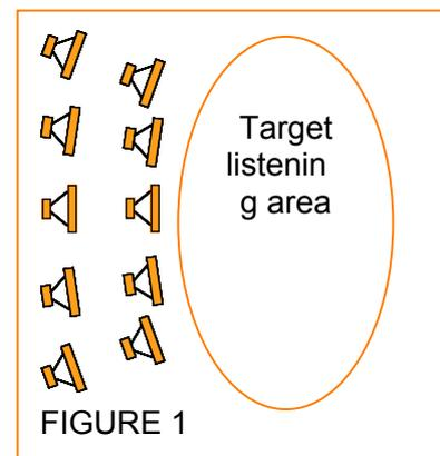
One interesting aspect of this approach is that if the reproduction reference is the vanishing point the loudspeaker arrays do not need to be accurately placed. The arrays are reproducing virtual source locations and so just need to align with each line from the vanishing point where sources are to be rendered and aimed to uniformly cover the target listening area.
